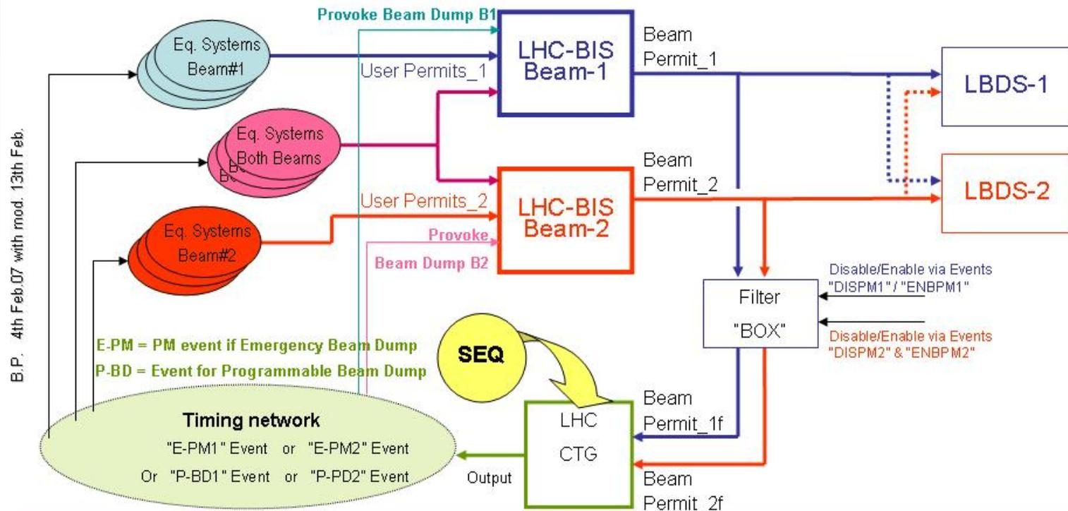
**In case of Emergency BD\*, the 2 beams will be always dumped thanks to a coupling between BIS-1 & BIS-2**
